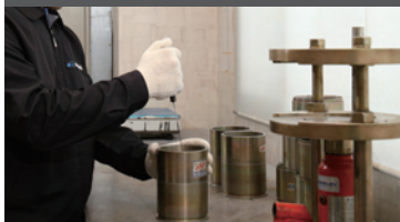
Mold to produce the specimens conforming to KS test standard
