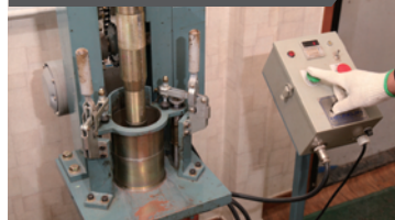
Equipment to compact the test specimens conforming to KS test standard
