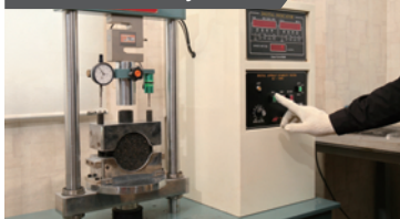
State-of-the-art digital equipment that can measure stability and flow values according to the KS test standard
